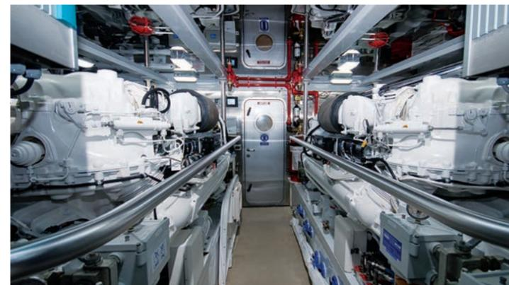
A pair of massive 2,600 hp MTU M94 diesels occupy the huge engine room and give the boat a top speed in excess of 35 knots.
