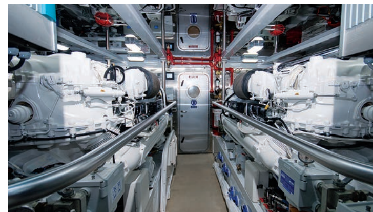
A pair of massive 2,600 hp MTU M94 diesels occupy the huge engine room and give the boat a top speed in excess of 35 knots.
